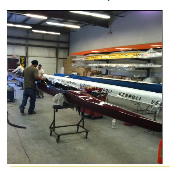
A rebuilt DM four with it's glossy paint is undergoing final assembly. Stretchers, tracks, seats and fin are being installed. All boats are rigged to be certain they meet factory tolerances.
