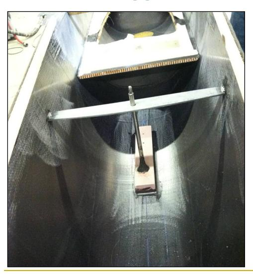
Here's a coxed four with the seat decks in and the rudder tube and fin support freshly bonded in place.
