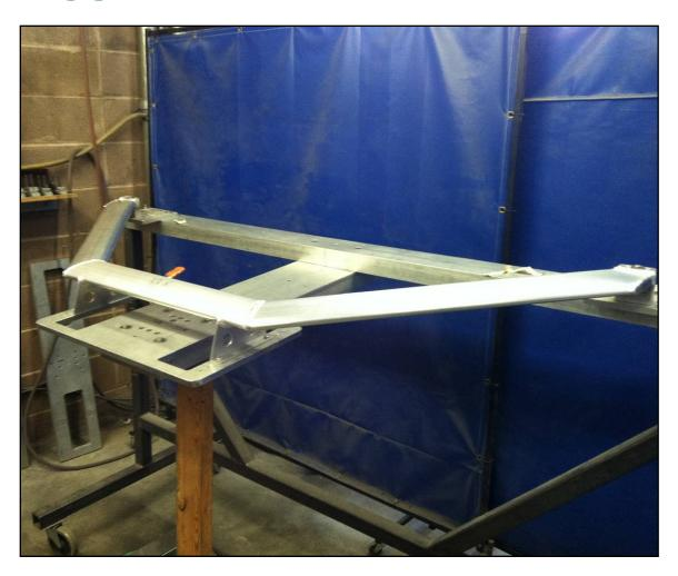
Riggers are manufactured in the welding shop. Here is a sculling wing rigger on the jig.
