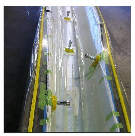
Here's a photo of a double that is vacuum bagged. The vacuum process causes the carbon fiber and honeycomb to bond and conform exactly to the shape of the mould, creating a very light and stiff structure.
