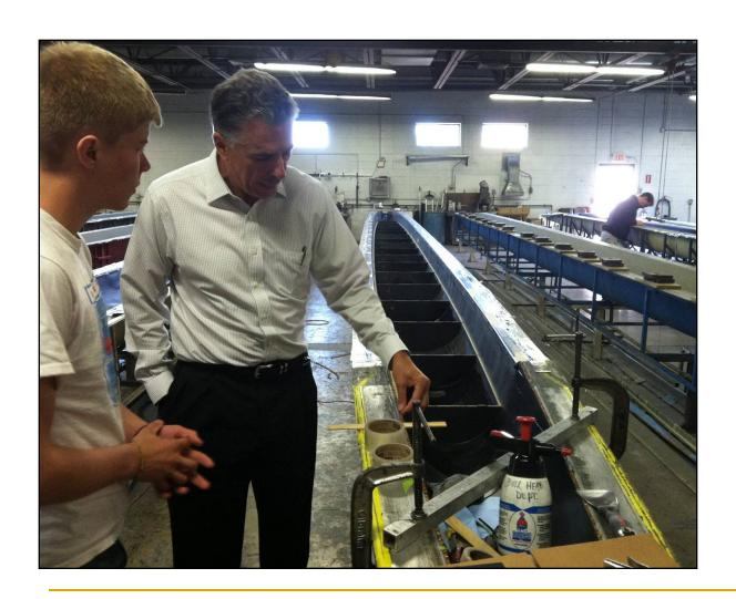
Once the boat has cooled and the oven removed, the bulkheads are bonded in and the boat has enough strength to be removed from the mould.
