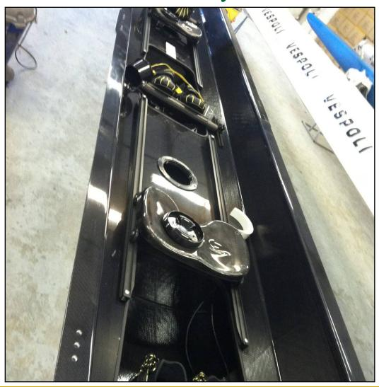
Here parts are being installed into the same four's refurbished hull.
