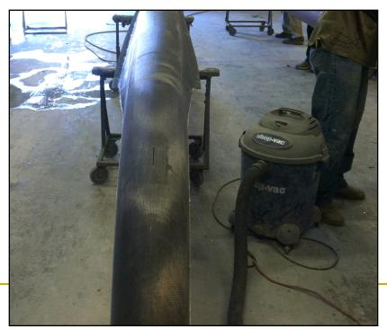
The upper boat is fresh from the mould. One can see the weave of the carbon cloth used on the exterior.
