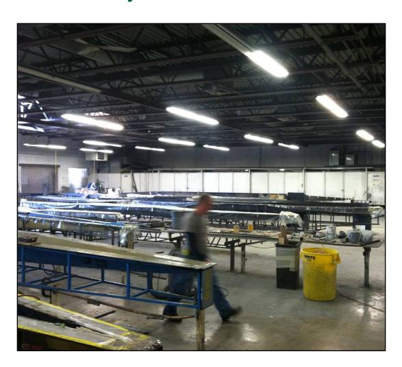
Each hull is laid up in the moulds you see here.
